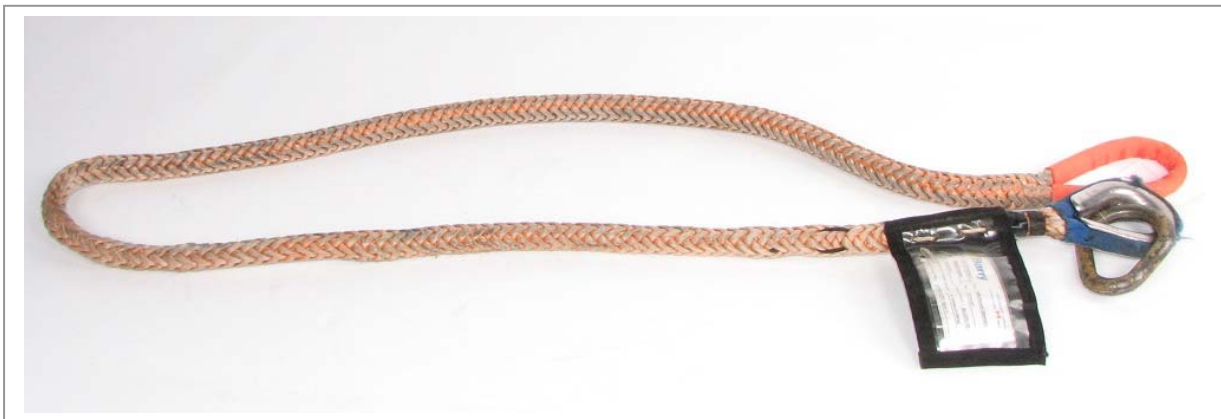
Figure 1 - Used longline spliced sample prior to break test
