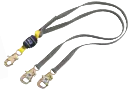
1246080 WrapBax™ 2 Tie-Back Lanyard Twin-leg with snap hook and 5,000 lb. (22 kN) WrapBax™ Hooks at leg ends x 6 ft. (1.8 m)
