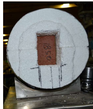
c) Projectile mounted in sabot
