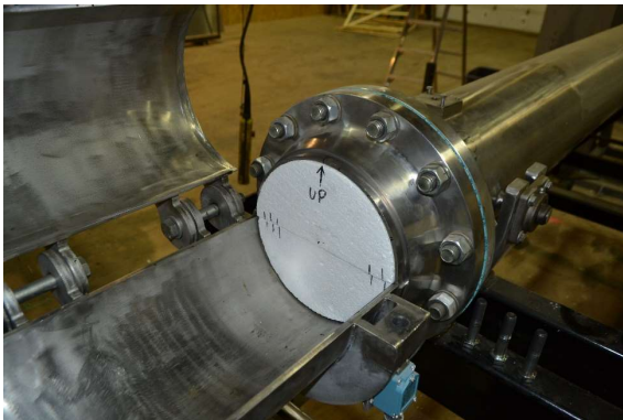
d) Loaded sabot mounted in breach
