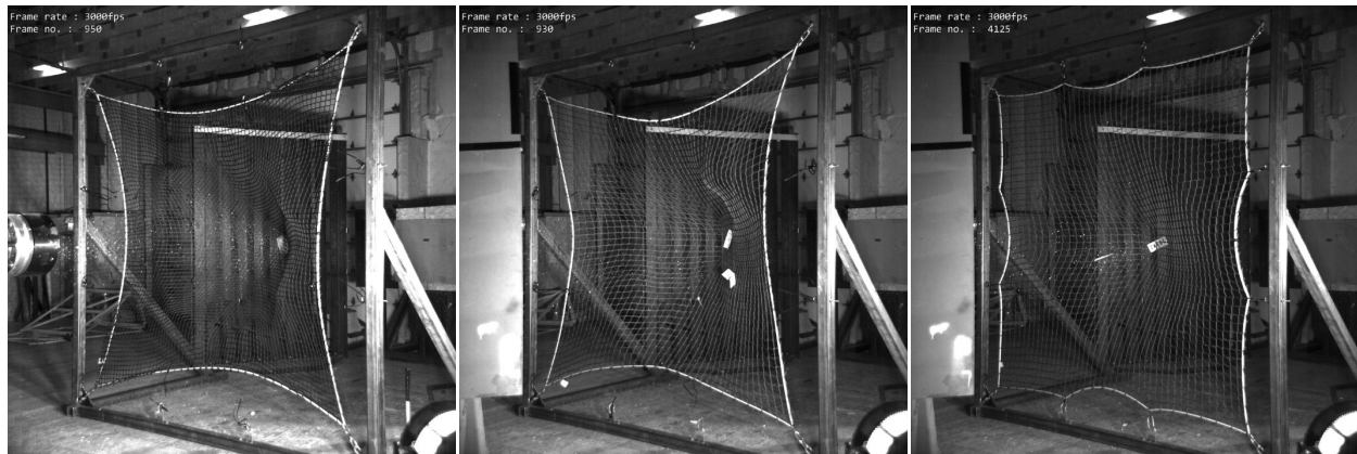
a) Test 3 FN700-1.5 with cable tie interior support at maximum deformation b) Test 6 FN700-2.5 with cable tie interior supports at maximum deformation c) Test 12 FN700-2.5 with rigid link steel interior supports at failure
